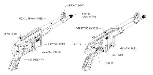
Operating controls are identical between all models of PLR-22 Pistol and SU-22 Rifle
