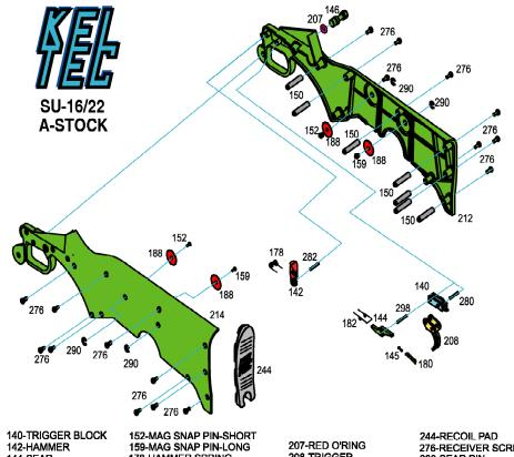
142-HAMMER 144-SEAR 145-SEAR SPRING PIN 146-SAFETY 150-SPACER-16
