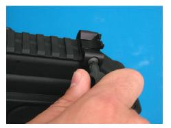
(not included) to depress the detent pin and turn the sight post by hand. One click (1/4 turn) will change the point of impact 1 inche at 50 yards. Clockwise moves the point of impact up and counter-clockwise moves it down.
