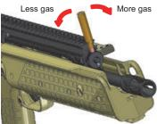
If the action is not ejecting a case, follow the unloading procedure. Then load a new full magazine and increase the gas until it ejects. Then increase gas one click for reliability.
