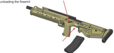
Insert a loaded magazine into the well behind the pistol grip. Make sure it is engaged by the magazine catch. Unfold the operating handle and pull it all the way back. Release the handle and let it go forward by its own power.
