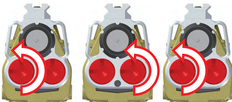
Unscrew magazine bolts with alternating 1/2 turns (KSG shown)
